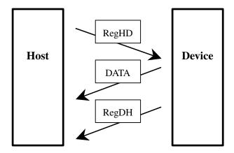
Figure 5.16 DMA data-in command protocol
